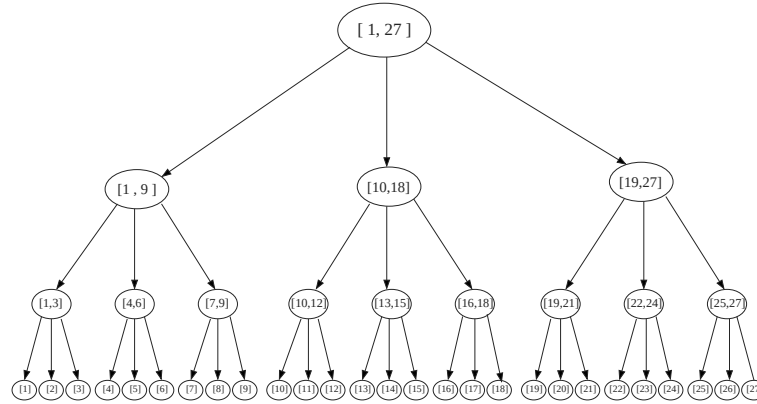
Fig. 1. The interval tree T for n = 3^3 , k = 3
